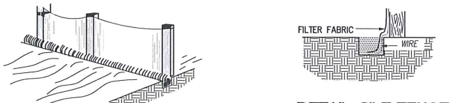
DETAIL: SILT FENCE NOT TO SCALE
