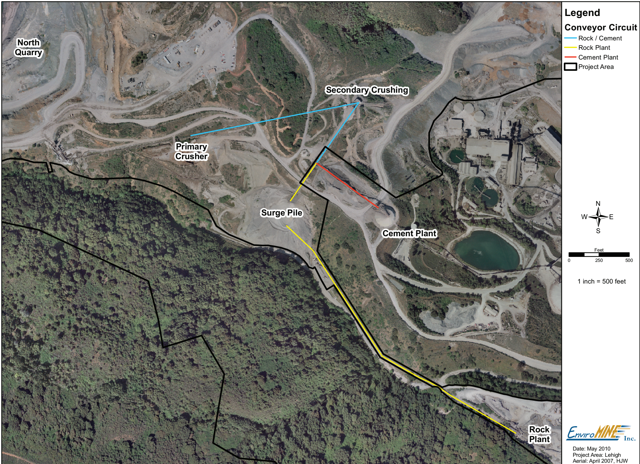
Figure 6 Quarry Conveyor Circuit
